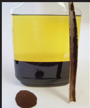
Ethanol damage encountered in the form of rust taken from the top of an injector, a rusted fuel line and a jar of phase separated fuel.
